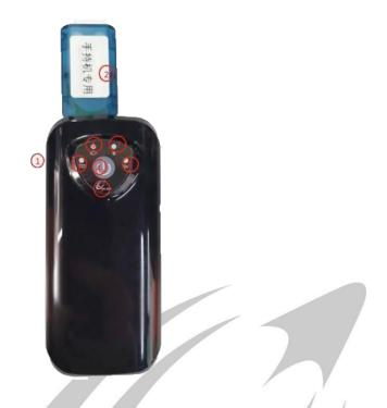
$(1)\,$  miniUSB charging input interface, the handheld can be charged through this interface.
