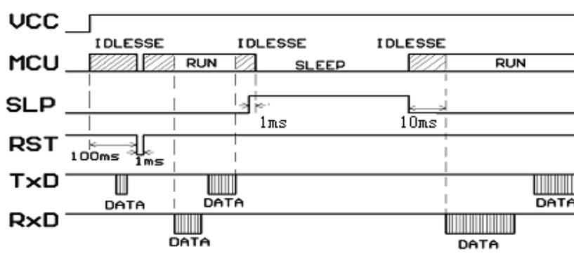
About the module without sleep function, users can cut off the power supply through electron switch to satisfy the power-saving purpose. When you use this method, pay attention to the connection signal level that connects with the external equipment and the time order relation, make the module achieve the minimum current consumption and ensure that the MCU isn't in the working state. The details are shown as follow:
