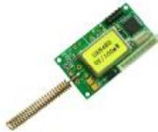
Our products can be embedded in users' equipment, if it doesn't have enough space to put the module, users can use the module with the spring antenna.
