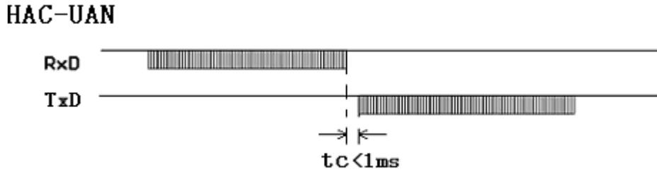
**b. The delay time of transceivers between the first byte sent by TxD and the first byte received by RxD.**
