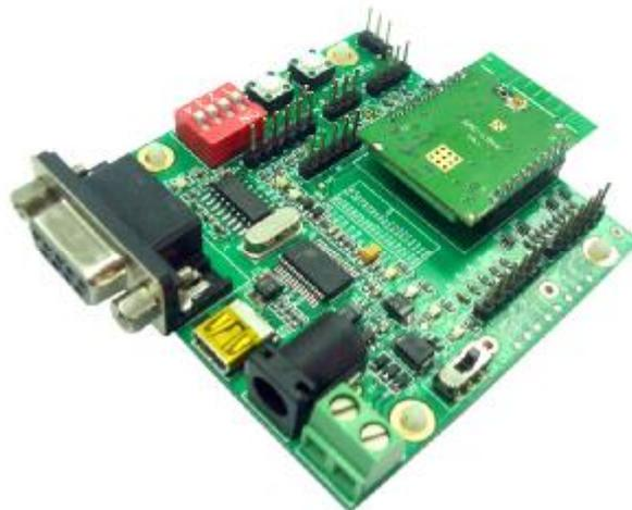
Picture 3 Connecting Methods between HAC-LBee V3.1-2.2 and HAC-DEV
