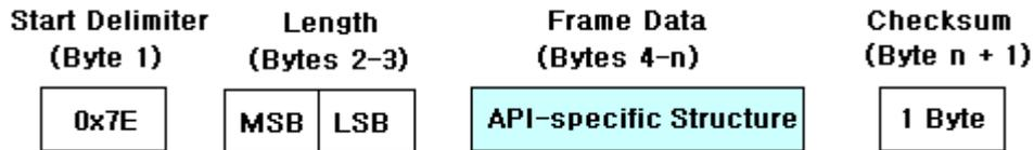
Every frame is composed of 4 fields, there are Start Delimiter, Length, frame data and Checksum.
