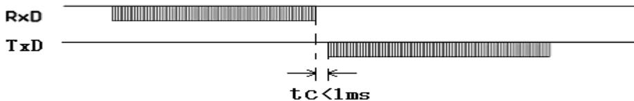
**b. The delay time of transceivers between the first bit sent by TxD to the first bit received by RxD.**
